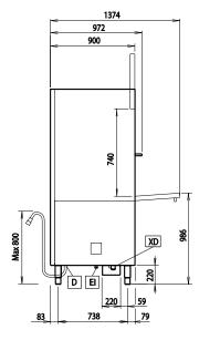
Drain ΕI Electrical inlet (power) EO HWI **Electrical Outlet** Hot water inlet ΧD Detergent connection
